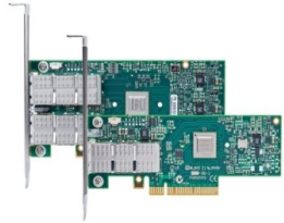
High Performance Interconnects – InfiniBand (with SR-IOV) <1usec latency, 200Gbps Bandwidth>
